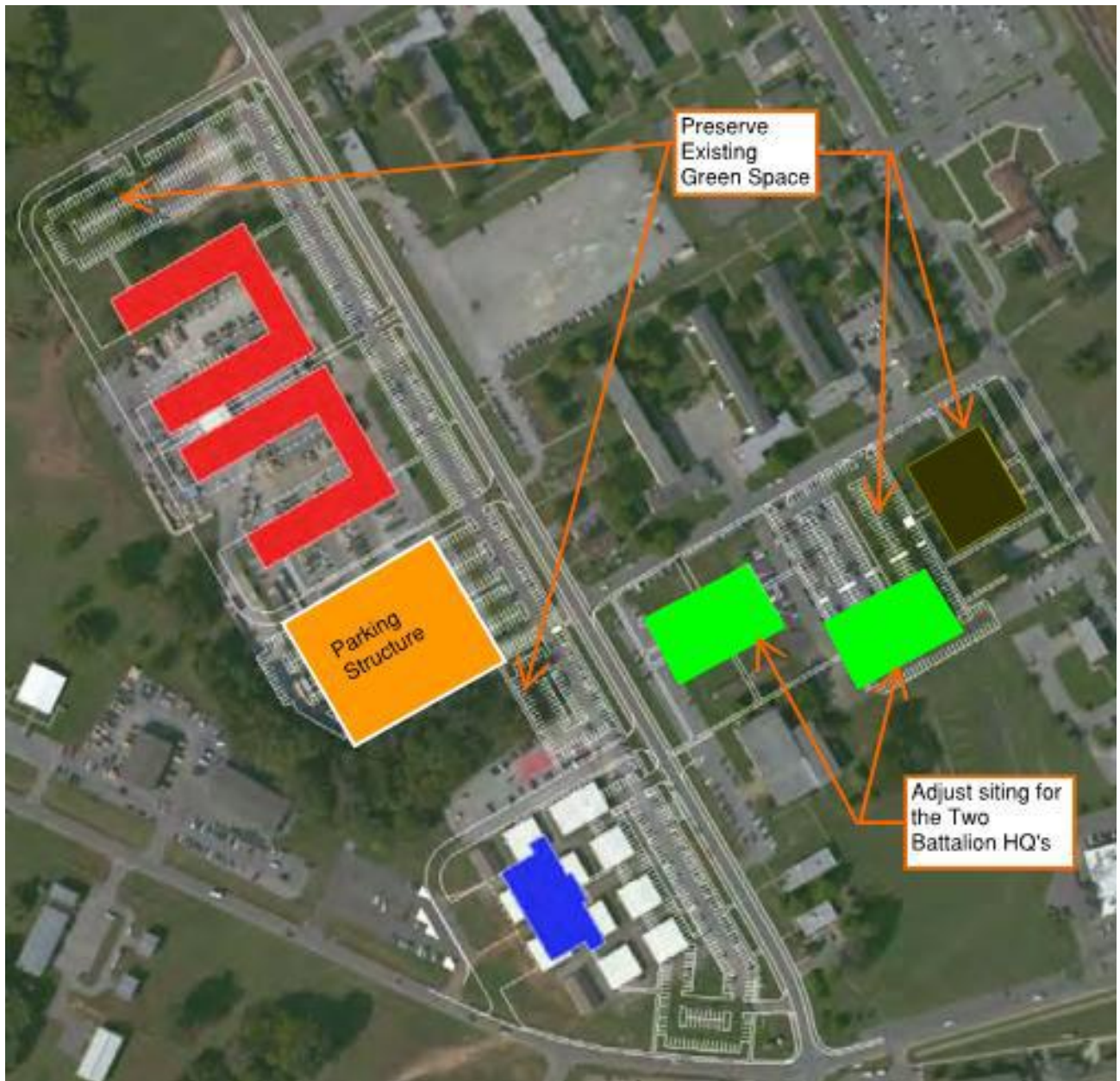
Proposed Location – 960 car parking structure (5-stories)
